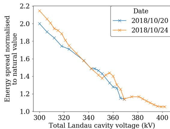
Figure 5: Measured energy spread in uniform fill at 149 mA in the 3 GeV ring as the total Landau-cavity voltage is increased.
