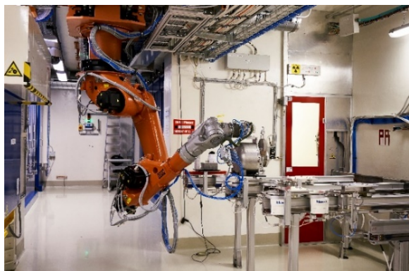
Figure 4: KUKA ® robot manipulating a MEDICIS target placed on the rail conveyor system (RCS).
