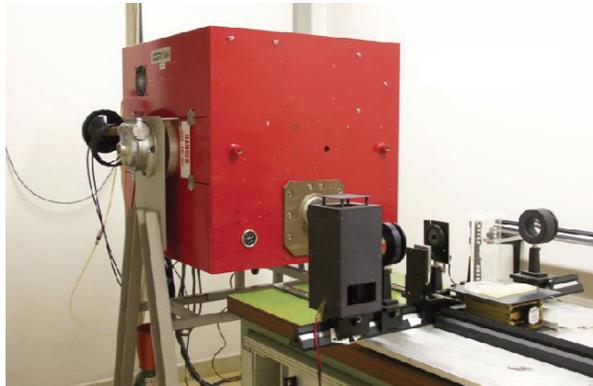
Figure 2: Kinetron accelerator.
